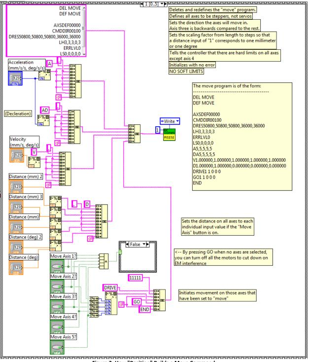
Figure 2: How "Position" Builds a Move Command
